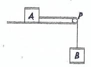
Initially the system is held at rest with the string taut. A horizontal force of magnitude 75 N is then applied to A in the direction PA so that B is raised. Find the magnitude of the acceleration of A and the tension in the string.
